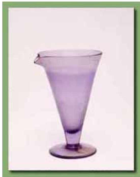
A glass flask used by Marie Curie during her research on radium. Radiation from the radium has changed the color of the glass.
